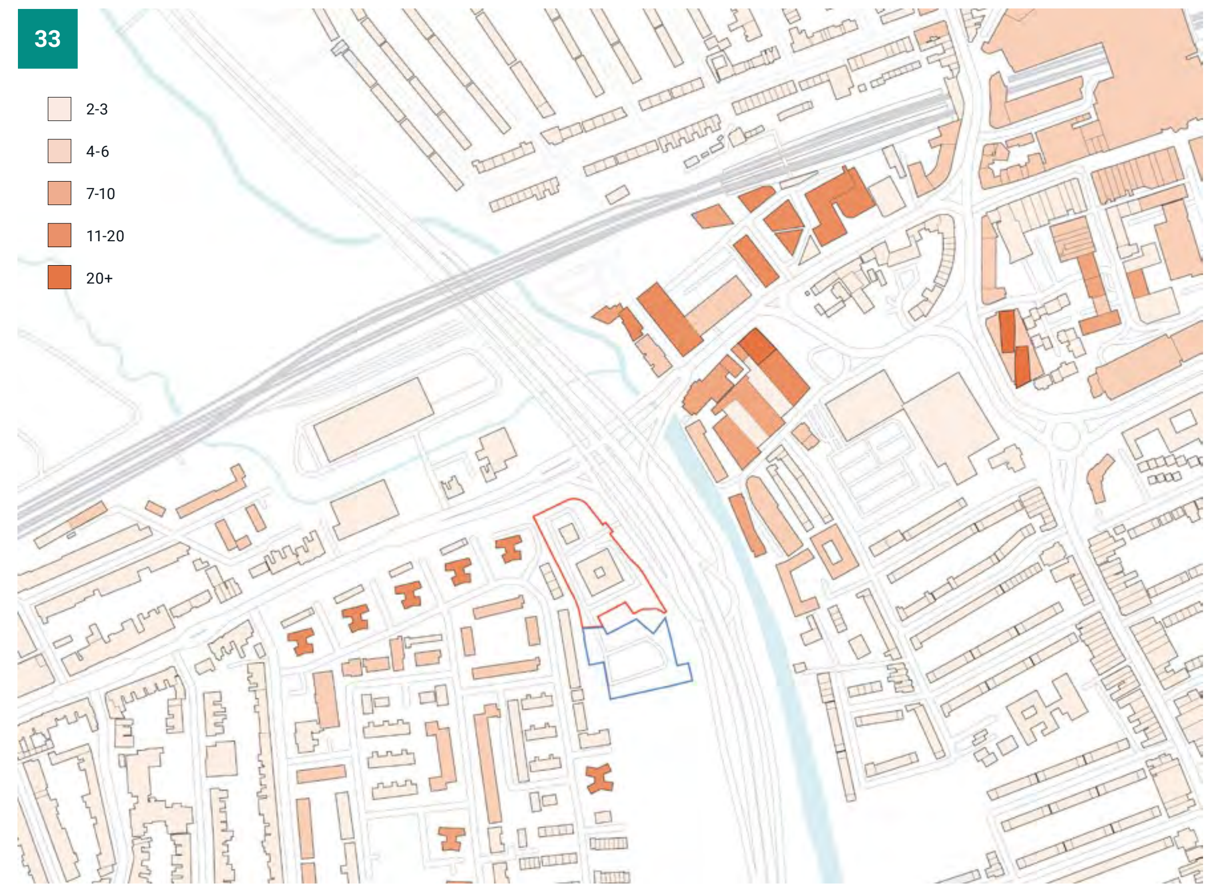
FIGURE 33 SURROUNDING HEIGHTS DIAGRAM The Analysis highlights the Concentration of Tall buildings along Romford Road and within Ilford Town Centre
