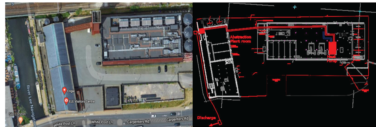
Figure 6: Heat pump solution within Kings Yard Energy Centre with abstraction and discharge points on the River Lea Navigation
