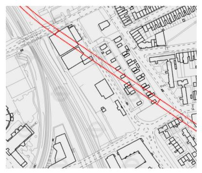
Plan showing approximate location of Central line tunnels in immediate vicinity of and potentially partially under site as red dotted line.
