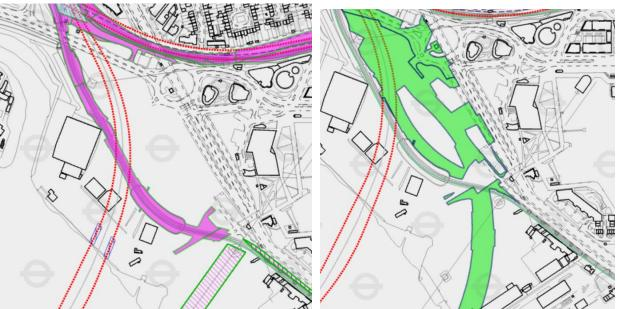
Plans showing approximate locations of LU Jubilee line tunnels under site as red dashed lines, DLR surface lines shaded purple, Cable car air space above site hatched purple and land acquired for Silvertown Tunnel surface works and tunnels shaded green.
